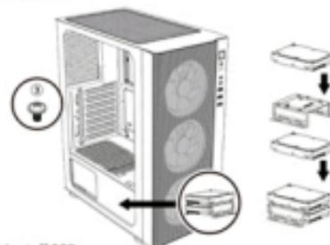
Hard disk enclosure for both SSD and HDD; unscrew hard disk enclosure and install HDD with screws.
