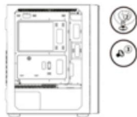
Please make sure that the motherboard aims at the copper cylinder and fix motherboard with No.3 screw.
