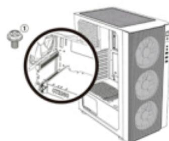
Remove the baffle marked in the picture, make sure the Graphic card aims at the motherboard slot and then fix Graphic card and case with No.1 screw.
