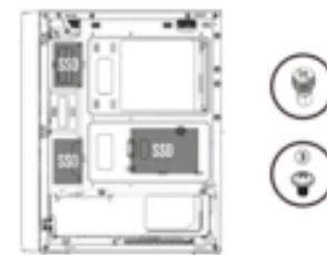
Hard disk enclosure for both SSD and HDD; unscrew hard disk enclosure and install HDD with screws.
